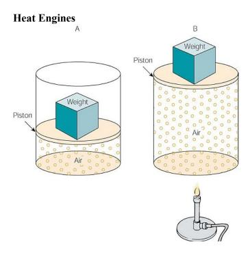
A **heat engine** is a device that converts heat into mechanical energy or work. This picture shows a very simple heat engine. The air in (B) has been heated, increasing the molecular motion and thus the pressure. Some of the heat is transferred to the increased gravitational potential energy of the weight as it is converted to mechanical energy.
