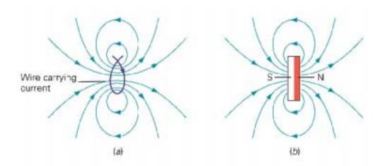
Forming a wire into a loop causes the magnetic field to pass through the loop in the same direction. Notice that all sides of the loop, by using the right hand rule, push the magnetic field the same direction. This gives one side of the loop a north pole and the other side a south pole. The magnetic field of the loop is the same of that as a bar magnet.
