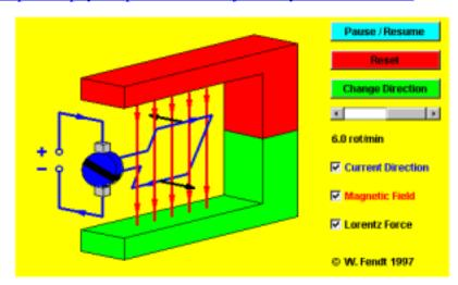
An **electric motor**, is a machine which converts electrical energy into mechanical (rotational or kinetic) energy. A current causes the coil to rotate mechanically. For this to occur
