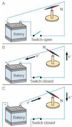
Oersted discovered that a compass needle below a wire (A) pointed north when there was not a current, (B) moved at right angles when a current flowed one way, and (C) moved at right angles in the opposite direction when the current was reversed.
