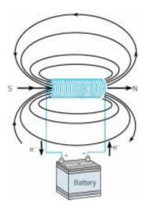
When a current is run through a cylindrical coil of wire, a solenoid, it produces a magnetic field like the magnetic field of a bar magnet.
