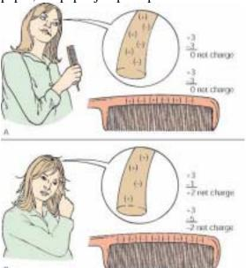
While I was in the bathroom I grabbed a small bit of toilet paper. As I brought the comb toward the paper, the paper jumped up and stuck to it. Why? The negative charges on the comb repelled the electrons in the paper. This left the positive charges near the comb. The negative comb and the positive side of the paper attracted each other and the paper stuck to the comb
