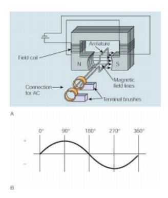
(A) Schematic of a simple alternator (ac generator) with one output loop. (B) Output of the single loop turning in a constant magnetic field, which alternates the induced current each half cycle.
