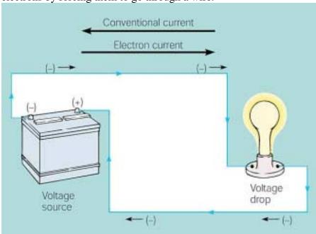
We can see the effects of this electron flow with the light bulb, which converts some of the energy of this movement to light. The light bulb also gets hot so it is converting some of the energy to heat. Light bulbs and heating elements are examples of resistors, they impede the flow of electrons. The flow of electrons is called **current** and is measured in amperes (A). An **ampere** is equal to a flow of 1 coulomb/second.
