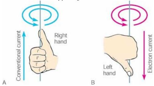
Use (A) a right-hand rule of thumb to determine the direction of a magnetic field around a conventional current. Remember that most people write current going from positive to negative. If your stubbornness requires you to thing about electron flow, you will have to reverse everything and use the left-hand rule of thumb.
