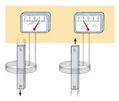
In the above picture, a current is induced in a coil of wire moved through a magnetic field. The direction of the current depends on the direction of motion. These induced currents only exist as long as the magnet is moving, and will die off when the magnet becomes stationary.
