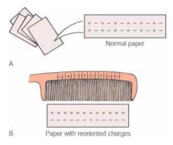
Charging by induction. The comb has become charged by friction, acquiring an excess of electrons. The paper (A) normally has a random distribution of (+) and (-) charges. (B) When the charged comb is held close to the paper, there is a reorientation of charges because of the repulsion of the charges. This leaves a net positive charge on the side close to the comb, and since unlike charges attract, the paper is attracted to the comb.
